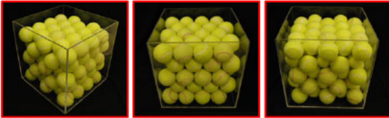
Figure 2 Image of a transparent box with tennis balls stacked inside in an orderly manner forming a type of crystal structure. The structure formed is bcc in this case.
