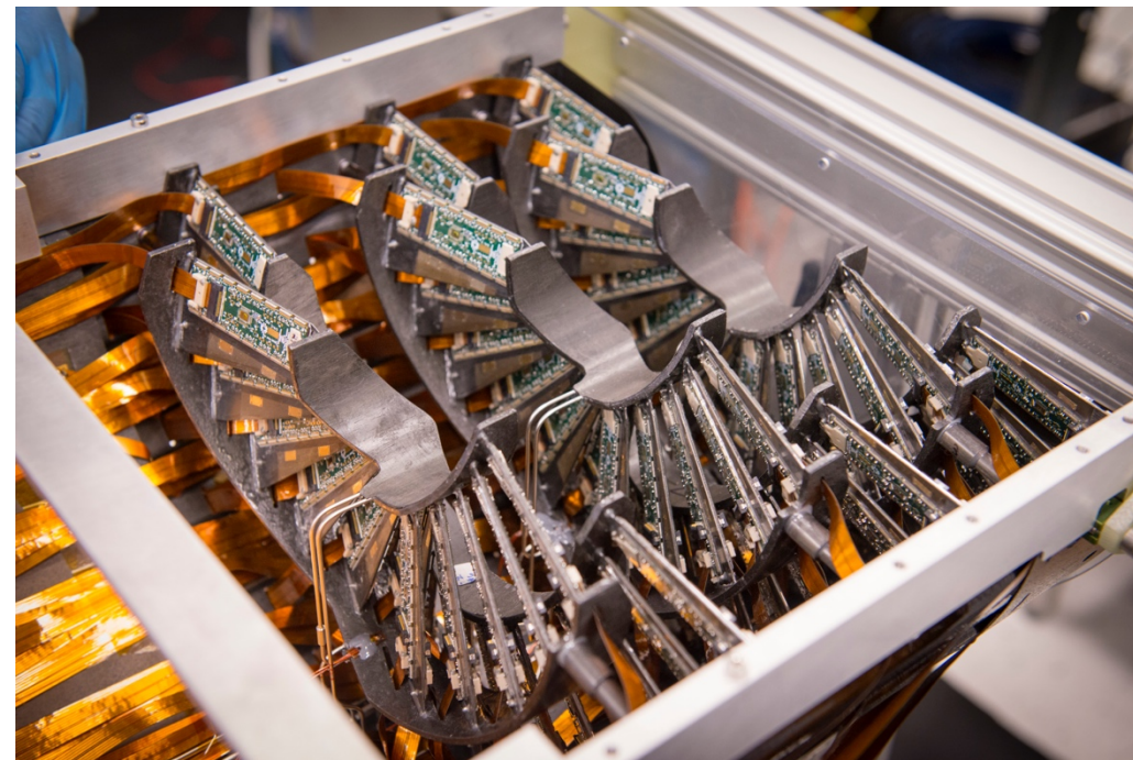
Half endcap disks for the upgraded CMS pixel detector, installed early 2017
