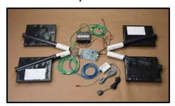
**Kit Contents:** 4 "counters" and photomultiplier tubes, power box, DAQ, GPS antenna and temperature sensor which can be placed outside. The DAQ creates a formatted message that can be sent to a computer and collected in a text data file through a USB interface. Computer commands set parameters for each experiment, monitor the data stream & display parameter settings and other important information.
