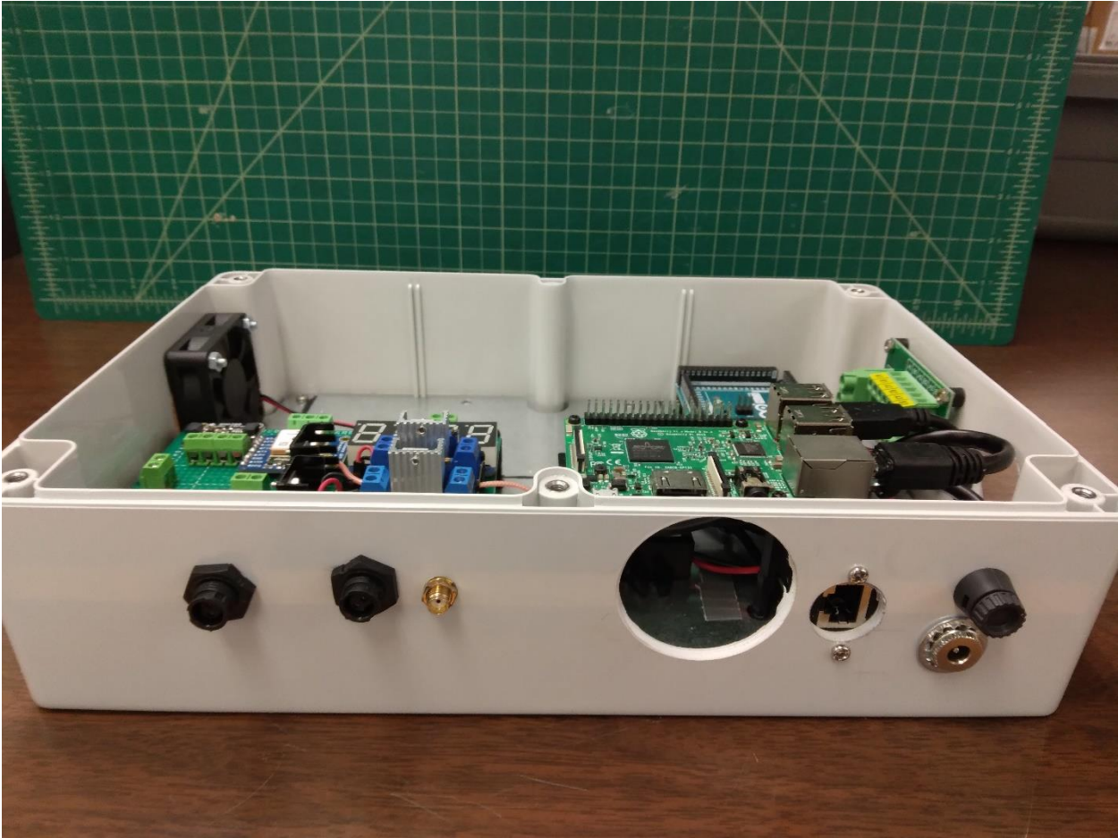
Rear side of the enclosure with all the connectors mounted
