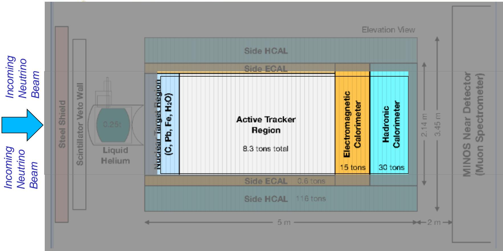
Muon neutrinos hit the carbon target. MINERvA measures the products of the interaction.
