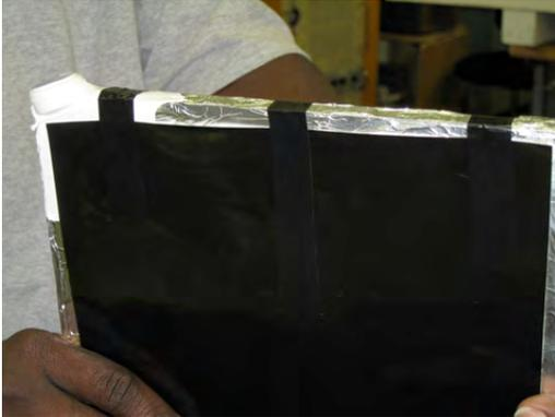
Use Teflon plumber's tape to wrap the edges of the cookie to block light; do not cover the face. Avoid scratching the face of the cookie. This is the transmission window for the light pulses.
