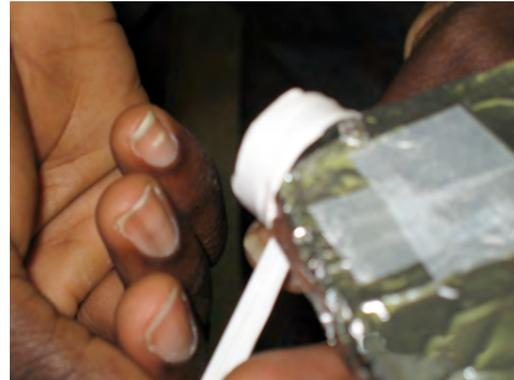
Completely cover the scintillator. While minor wrinkles are acceptable, avoid holes or tears. Add additional “repair” pieces to patch any noticeable tears or holes.
