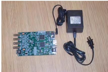
1. Power Supply, female connector → DAQ male jack (power supply may differ from photo)
