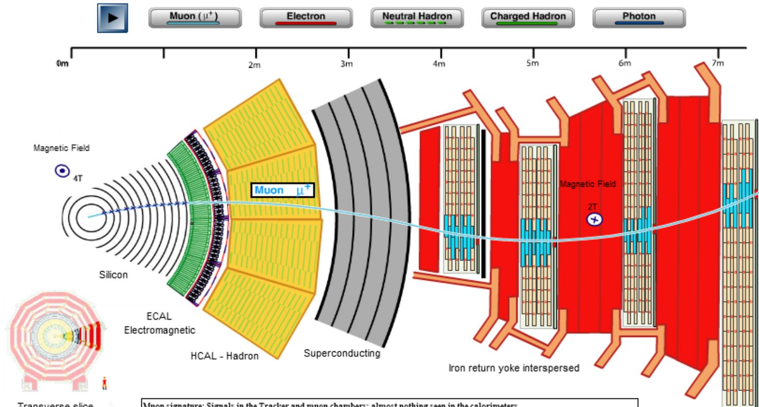
**Muon signature:** Signals in the Tracker and muon chambers; almost nothing seen in the calorimeters. Muons are perhaps the easiest particles to identify in CMS: no other charged particle traverses the whole detector. Being charged, they are bent by the field in one direction inside the solenoid and in the opposite direction outside. As muons can only arise from the decay of something heavier their presence signifies that something potentially interesting has happened.
