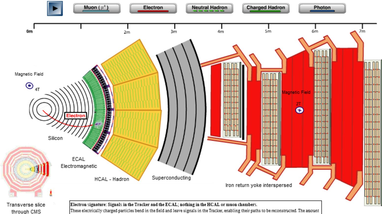
**Electron signature:** Signals in the Tracker and the ECAL; nothing in the HCAL or muon chambers.
