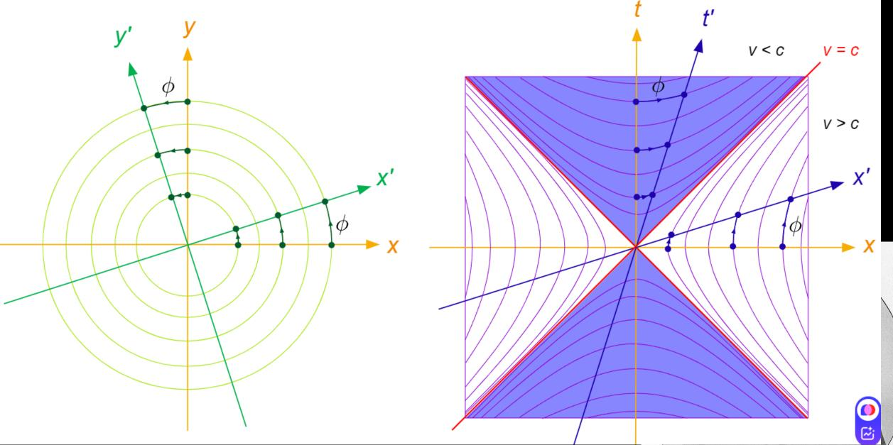
This makes spacetime hyperbolic not circular. The hyperbolas sections show that an observer can't catch up to a light beam.
