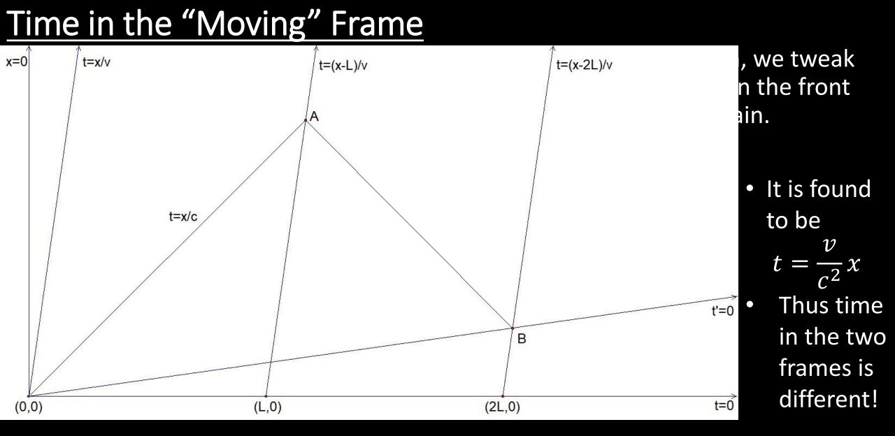
• If we can find the coordinates of point B, we can find the line of simultaneity of the flashlights for the train observer in the coordinates of the ground observer.\*
