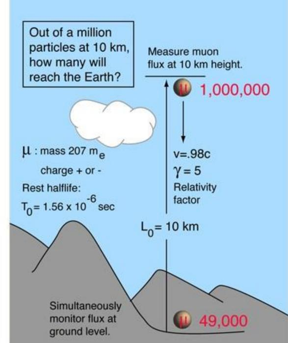
Distance:  $L_0 = 10^4$  meters 2000 m Time: T = (0.98)(3 x 10<sup>8</sup> m/s)  $T = 6.8 \times 10^{-6} s = 4.36 halflives$ Survival rate: -4.36= 0.049Or about 49,000 out of a million. The muon sees distance as length-contracted so that  $L = L_0 / \gamma = 0.2 L_0$ = 2 km.
