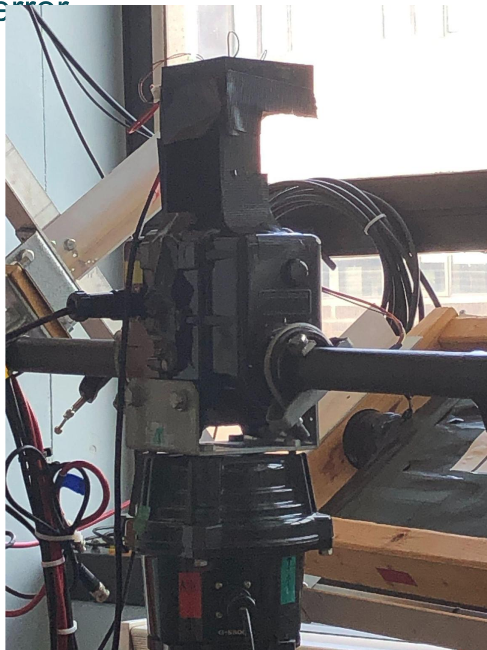
The Imu Sensors mounted upon horizontal Rotator
