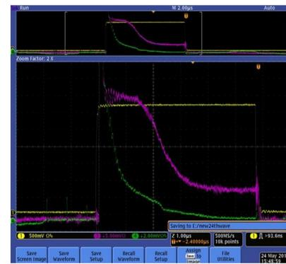
In the above oscilloscope traces the smoother red line represents the 300 micro seconds that an LED light bulb was on; the choppy white line represents the PMT response signal. Clearly the PMT detected the light for the entire time it was on. The PMT was a SensTech model used with QuarkNet cosmic ray detectors.
