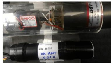
A photomultiplier tube detects these very faint light flashes of light by transforming the light via the photoelectric effect into an electrical pulse which is sent to a data acquisition board for signal selection.
