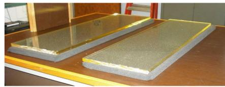
Scintillator is made of PVT plastic doped with fluorescent hydrocarbon molecules. When a charged muon goes through the scintillator it ionizes plastic molecules causing them to emit photons of UV light. The hydrocarbons absorb UV and re-emit green light which is detected by a photomultiplier tube. The plastic is wrapped with foil to prevent loss of light and with black paper to prevent outside light from getting in.
