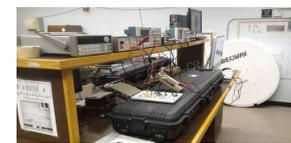
The black enclosure houses a 1 meter long cosmic ray detector built by students in QCC's physics lab; the enclosure protects it from ambient light
