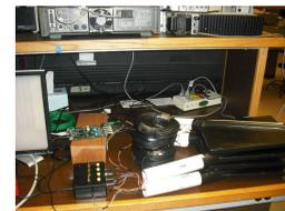
Three QuarkNet scintillator detectors are shown wrapped in black, and the DAQ. The PMTs are within the white PVC tubes
