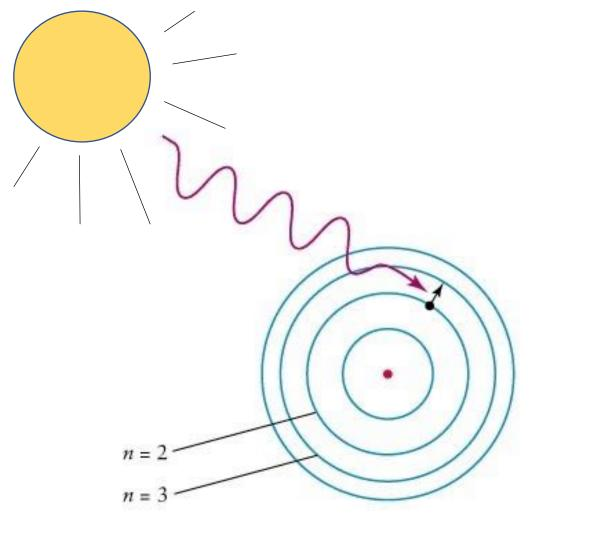
Atoms and molecules absorb light at very specific wavelengths, leaving a "chemical signature"
