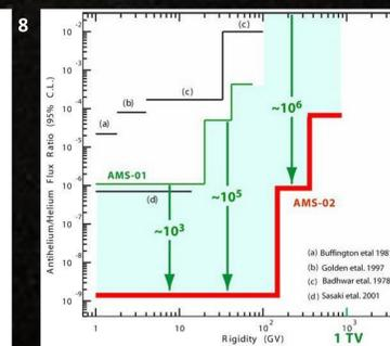
The AMS-02 Detector (left) will analyze the helium/antihelium flux of the universe with a sensitivity of  $10^{-9}$  (above).
