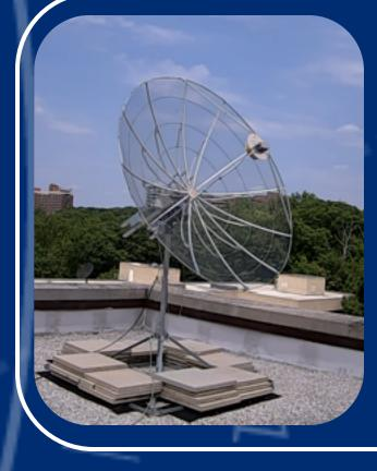
Data Collection Using JHU's 2.5 m Small Radio Telescope (SRT), I collected 10 days worth of data. The C script written by MIT to operate the SRT outputted the raw frequency spectra and relevant variables into a .rad file.
