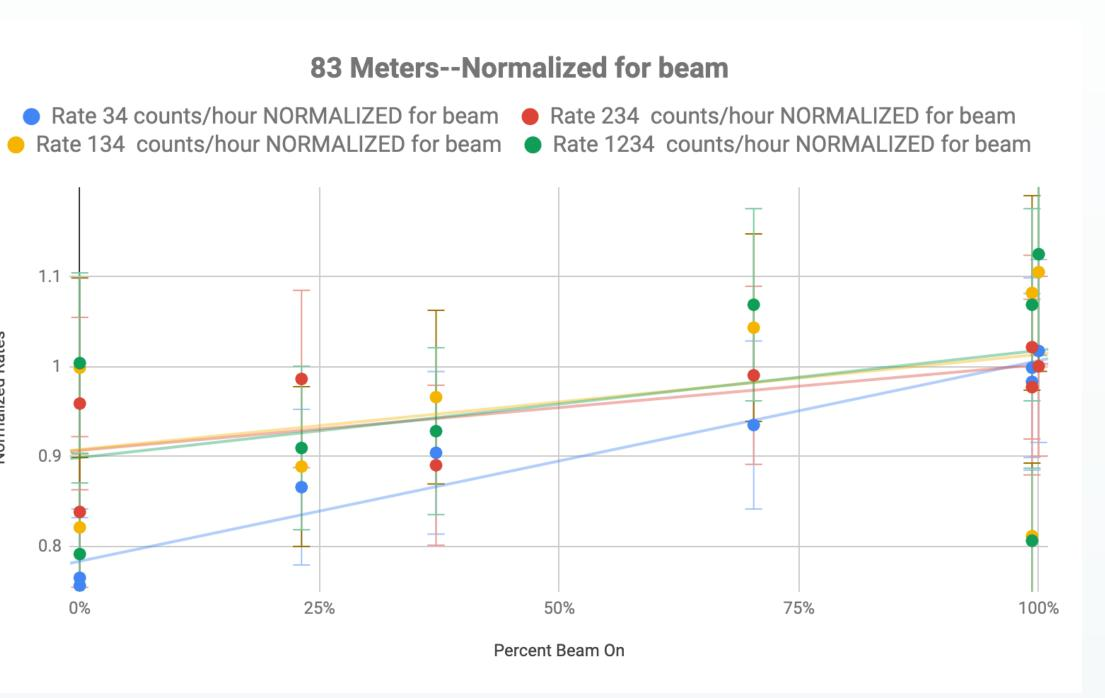
Figure 5. Normalized cosmic ray muon rates as function of percent beamline on; rates increase as percent beam increased, indicating the need for corrections in the rates.
