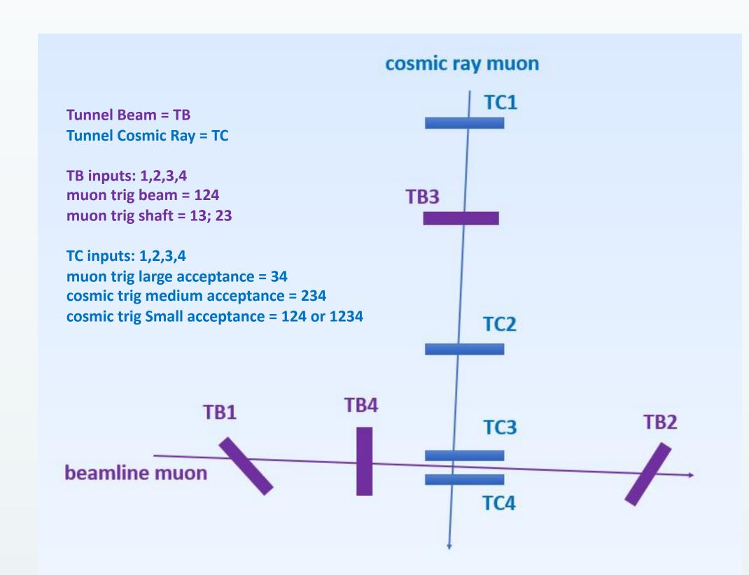
Figure 1. Diagram of underground setup. TC is the vertical cosmic ray muon detector, while TB is the horizontal beamline detector.
