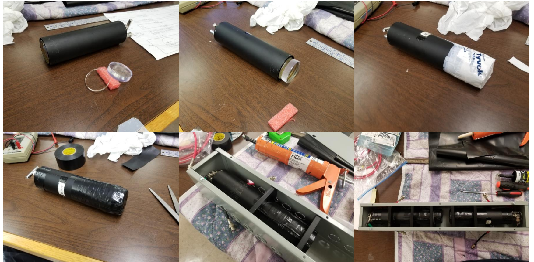
Figure 13: Top left to bottom right: Assembling the BC-408 scintillation counter and installing it into the prototype housing. The NaI(Tl) scintillation counter was assembled in a similar process. Both are shown in the housing at bottom right. Brackets were custom-designed and 3d printed.
