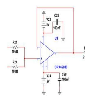
The Adder subcircuit takes in the two signals from their respective shapers an sums their averages, generating one output signal. It has a gain of 1 and does not invert the output signal.
