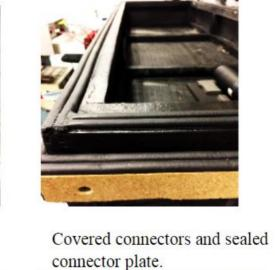
and installing the additional wood liners and gasket, DYNAFLEX 230 black silicon was used to fill in all corners, gaps on the inside and outside of the box. The box was measured to be 92% light tight. The leaks were found to be through the bulkhead connector panel. DYNAFLEX 230 black silicon was used to fill around all SHV and BNC connector interfaces through the metal bulkhead panel, and the unused bulkhead connectors were covered, after the box was measured to be 99.6% light tight.
