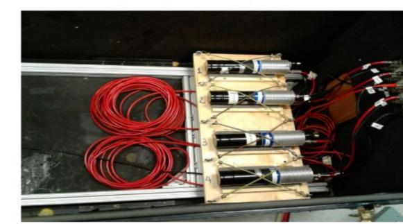
PMTs with high dark rate were rejected. Of the 77 Hamamatsu PMTs that were tested, 15 of them were
