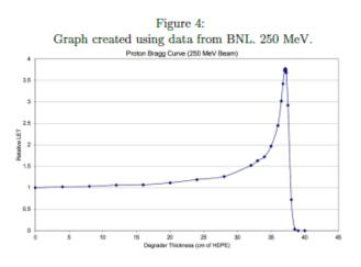
We found a close correlation between the measured Bragg peak depth (26.1 cm at 205 MeV and 37.1 cm at 250 MeV) and our calculated values (26.33 cm and 34.67 cm, respectively).
