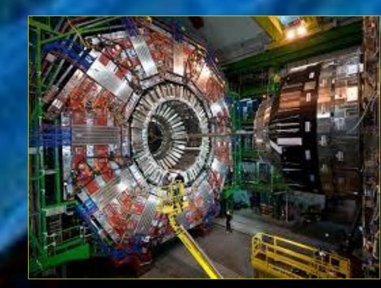
•CMS machine, 13,800 tons, 52 feet in diameter, 70 feet long, 100 million different detection elements.
