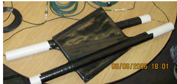
Figure 15. The latest version of the cosmic ray counter consists of scintillator, cookie (the flat paddle region), PVC pipe support (white cylinder, partially wrapped in black tape), and the PMT (black wrapped portion of the PVC pipe).
