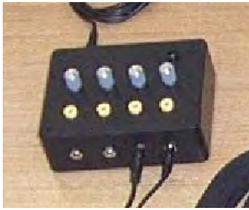
Figure 14. Power distribution unit. One black and four yellow test points allow one to check voltage on the PMTs.
