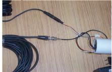
4. PMTs/counters BNC connections (4) ←→ DAQ BNC connections: 50 ft. BNC signal ext cables
