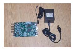
1. Power Supply, female connector  $\rightarrow$  DAQ male jack (power supply may differ from photo) Note: Do not plug into wall outlet at this step.
