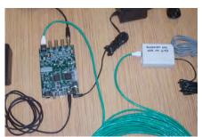
5a. GPS antenna → GPS Receiver Assembly: black MCX cable
