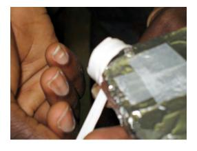
Completely cover the scintillator. While minor wrinkles are acceptable, avoid holes or tears. Add additional "repair" pieces to patch any noticeable tears or holes.
