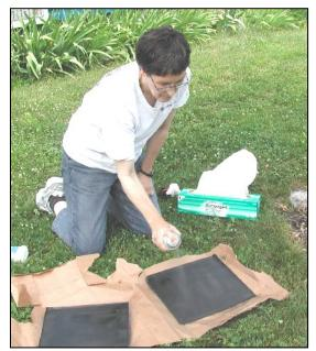
Finding a strong, flat black paint might be difficult. Also the paint may bubble and peel after repeated usage under extreme conditions. One alternative is to use artist's black paper on the bottom of the chamber. The paper lies flat on the chamber, and can be lifted out to dry after each viewing session.
