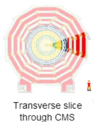
**Muon signature:** Signals in the Tracker and muon chambers; almost nothing seen in the calorimeters. Muons are perhaps the easiest particles to identify in CMS: no other charged particle traverses the whole detector. Being charged, they are bent by the field in one direction inside the solenoid and in the opposite direction outside. As muons can only arise from the decay of something heavier their presence signifies that something potentially interesting has happened.
