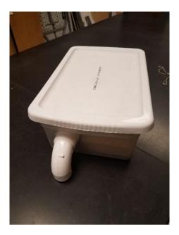
Cut a 2 3/8" hole in the flat end of the plastic box, high enough so that there is clearance of the bottom of the 2"  $90^{\circ}$  PVC (or  $45^{\circ}$ ) street elbow. Place a 2"  $90^{\circ}$  PVC (or  $45^{\circ}$ ) street elbow at the hole, and anchor it with a 2" coupling or male adapter or coupling on the inside of the box. White glue is sufficient.
